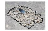
A minimum 500 mm (20 inch) diameter, **new** Corrugated Steel Pipe culvert is required
